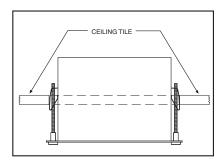
c. Compress the spring clips on the back box and push it through the hole, until the clips spring back. Tighten the screws until you hear a clicking noise. d. Attach the wiring to the circuit board inside the back box. When finished, close the door to the back box and turn on the power. The red LED will light.
